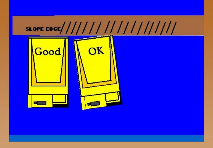
> "OK" shows the rear wheel on the driver's side making contact first. The driver should have a good view of this and stop before hitting or over-traveling the berm.
